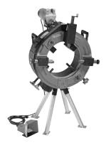
Includes riser blocks and grooving heads for cut grooving 4 – 12" ductile iron rigid groove. Power drive supplied requires 120 volt, 11.5 amp electrical supply. Stand included at no extra charge.
