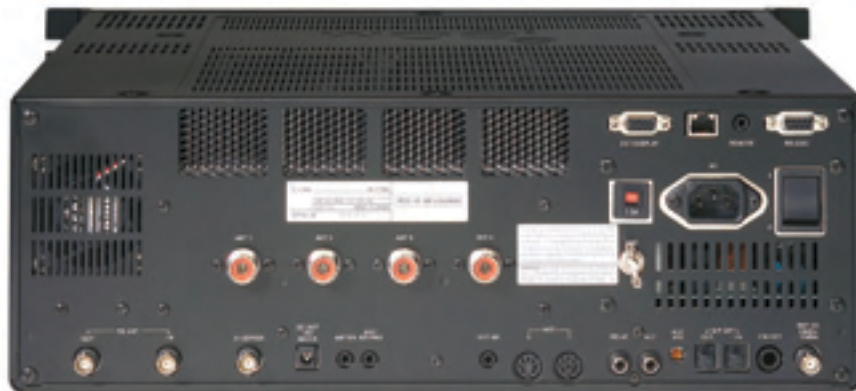
Figure 4 — The rear panel of the IC-7700 includes four antenna connectors, provisions for a separate receive antenna or preamp, and various accessory connections.
