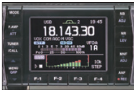
Figure 1 — The IC-7000 display screen is small, but the incredible resolution and use of color make it easy to see and use.
