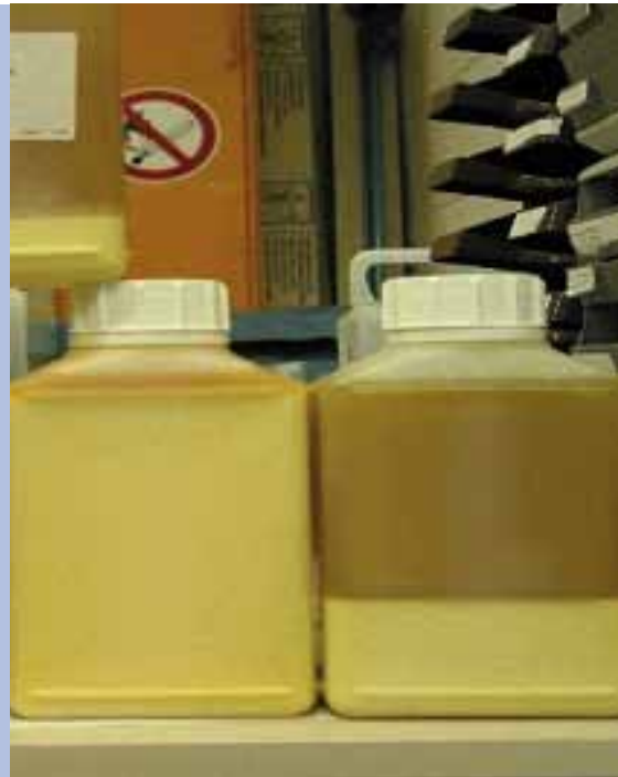
Loss of viscosity, phase separation and sedimentation due to microbial thickener degradation
