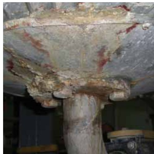
Bacterial growth on the base of a formulation vessel. With the appropriate plant hygiene, this can easily be avoided.
