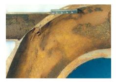
When the corrosive attack is generated on a metallic surface due to the flow velocity and producing mechanical wear, this is called erosion.
