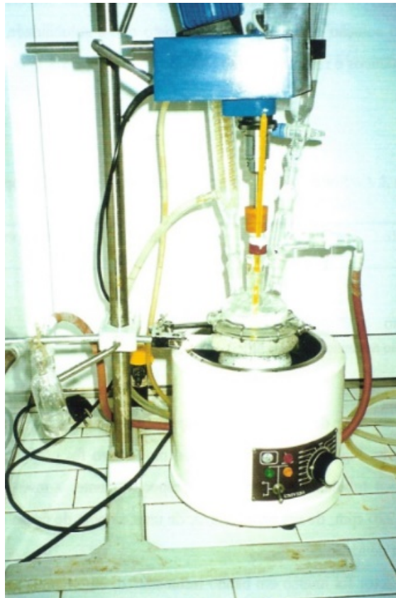
Scheme SM 16.2.1 – The apparatus for the synthesis of the copolymer
