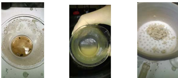
Figure SM 16.3.3: (A) Honey colored adipic acid (B) crystallization from hydrochloric acid solution and (C) product filtration.
