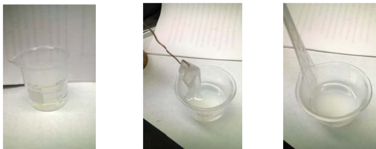
Figure SM 16.3.7: Adipoyl chloride and basic diamine solution (2 phases) and removal of Nylon strand using a copper wire hook.
