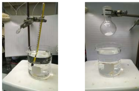
Figure SM 16.3.4: Reaction set-up before addition of oxalyl chloride.
