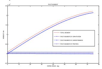
Fig.1. MLG actuation static loads
