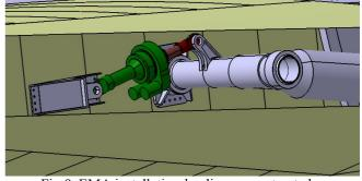
Fig.9. EMA installation-landing gear retracted The major components parameters and weight are listed in the table 5. The transmission takes most of the weight.
