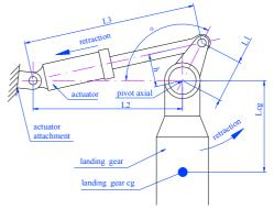
Fig.3. Landing gear kinematics
