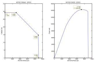
Fig.4. EMA Motor speed-torque and speed-power curves
