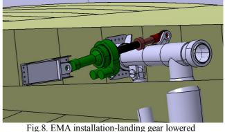
Fig.8. EMA instantion-failding gear lowered
