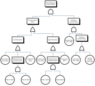
Fig.10.Fault tree analysis
