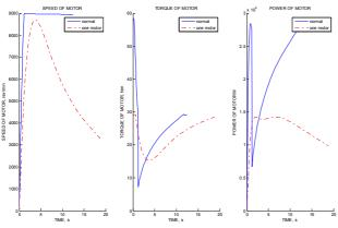
Fig.7. EMA motor dynamics
