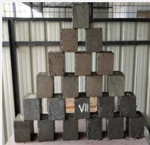
Figure 2. Test Specimens to measure compressive strength
