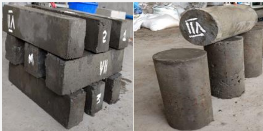
Figure 3. Test specimens to measure flexural and split tensile strength
