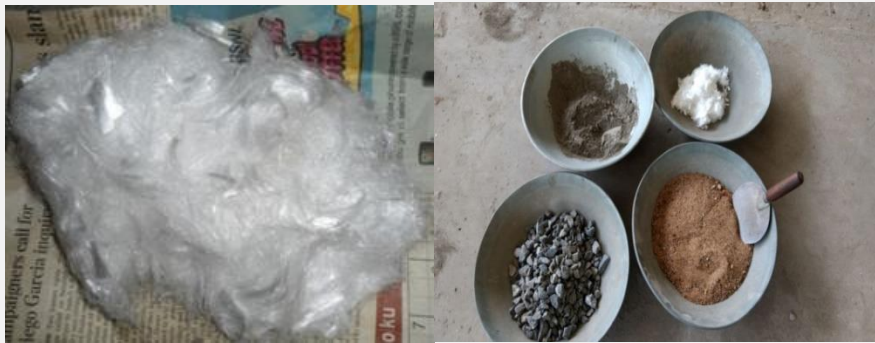
Figure 1. Polypropylene fibre and ingredients of concrete
