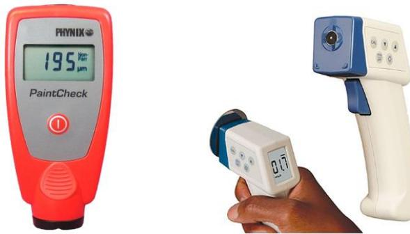
Figure 3: Digital Thickness Gauge (Shoe or Gun type)
