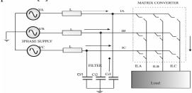
Fig. 1: General Architecture of Matrix Converter
