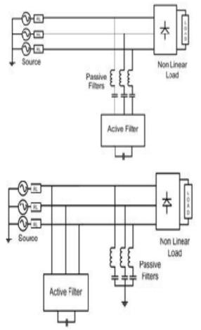
Fig. 2: Different structures of hybrid filters in power system
