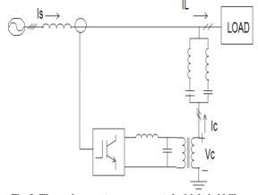
Fig. 3: Three phase system compensated with hybrid filter
