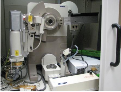
Stage and CCD sitting on base plate
