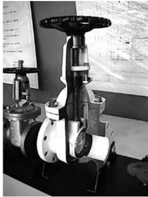
Fig. 3.7-3 Flanged end type (valve where the facing flange couplings are connected by tightening the gasket with bolts and nuts) 3
