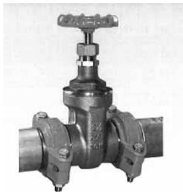
Fig. 3.7-5 Housing type (valve sealed with a rubber ring after grooved pipes are connected to prevent them from slipping off) 3
