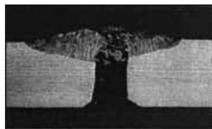
Insufficient penetration of welded area
