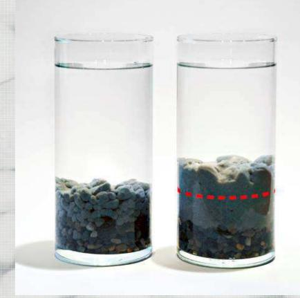
Extreme low-permeability (5x10<sup>-8</sup> cm/sec) result of consistent swell <u>and</u> self-compaction
