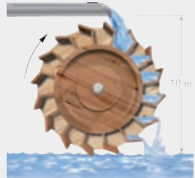
FIGURE 8.23 An overshot waterwheel.
