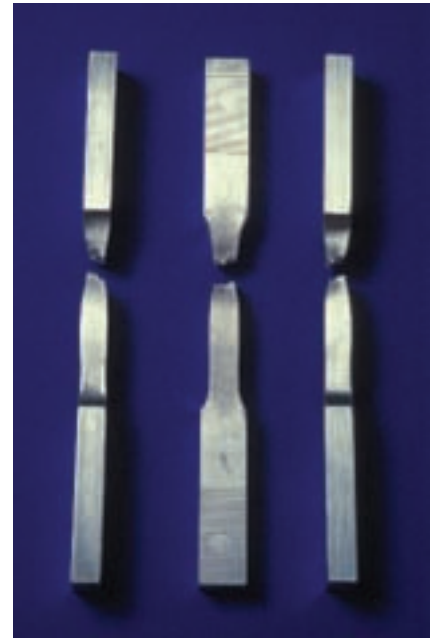
FIGURE 14.29 These rods of steel broke apart when a large tension was applied.
