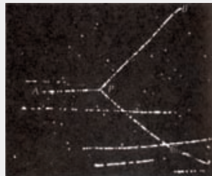
FIGURE 11.20 Elastic collision between two protons. The final velocities of the protons are perpendicular.
