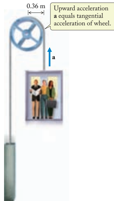
FIGURE 12.11 Elevator supported by a cable that runs over a rotating wheel.
