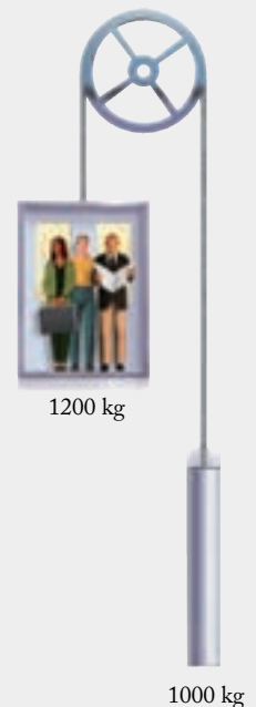
FIGURE 7.27 Elevator cage and counterweight.
