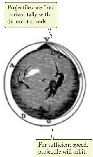
FIGURE 9.18 This drawing from Newton's Principia illustrates an imaginary experiment with a cannonball fired from a gun on a high mountain. For a sufficiently large muzzle velocity, the trajectory of the cannonball is a circular orbit.
