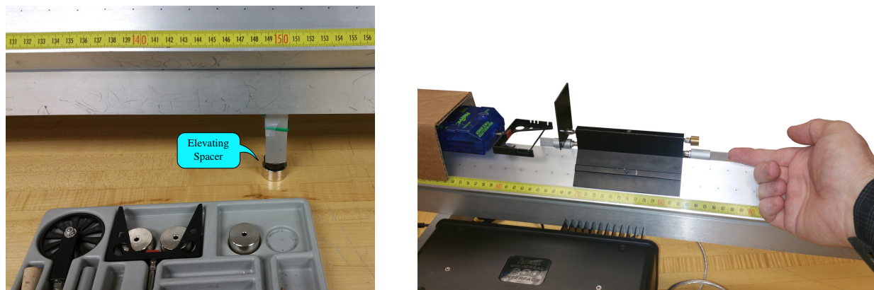
Figure 6.1: Before measuring the spring constant, remove the elevating spacer so the track is level. Execute the Hooke’s Law Capstone setup and slowly press the cart against the elastic rubber bumper. Slowly release the spring and stop Capstone. The motion sensor measures the cart position ( x ) and the force sensor measures the spring force F_s .
