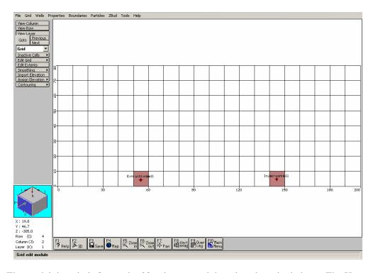
The model domain is 8 rows by 20 columns, and there is only a single layer. The X extent is 200m; Y extent is 80m.
