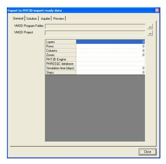
The **VMOD Program Folder** field allows the user to select the VMOD installation folder (by default the folder is C:\Program Files\Visual MODFLOW). This folder contains the VMOD.xml file which is required to locate the PHREEQC thermodynamic database.
