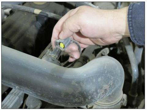
(Figure 3-1) Disconnect Intake Air Temperature Sensor (IAT).
