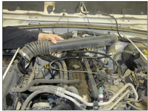
(Figure 3-3) Air Filter and Intake Tube Removal
