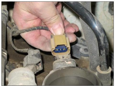
(Figure 3-6) Disconnecting the Throttle Position Sensor (TPS)
