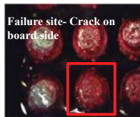
(a) Failure on board side
