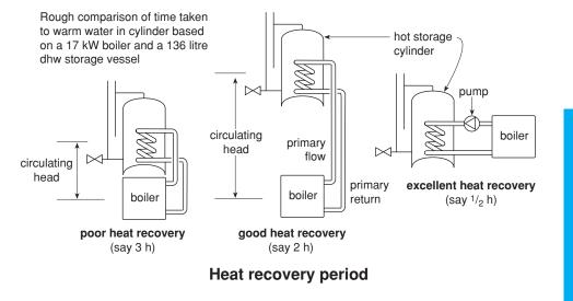
The heat recovery period is also influenced by the design and dhw cylinder used. All modern systems use BS 1566 cylinders. These have no less than 5–6 turns within the heat exchanger coil and the cylinder includes factory-fitted insulation foam. High performance cylinders can also be purchased with an even greater number of coils. The following chart shows the number of boiler cycles and approximate time required to raise a typical 136 litre cylinder up to the required temperature.
