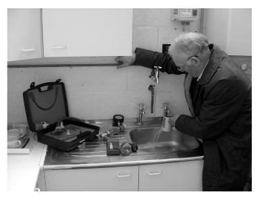
Operative taking water flow, pressure and temperature measurements
