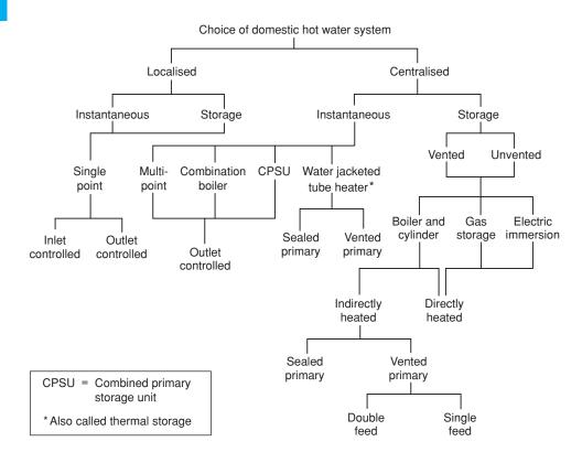
A localised system is one in which the water is heated locally to its needs, e.g. a single-point heater located above a sink. It may be chosen where a long distribution pipe would mean an unnecessarily long wait for hot water to be drawn off at the appliance.
