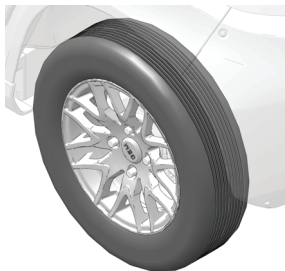
14-inch Cast Aluminum 63 lb-ft (85.4 Nm)
