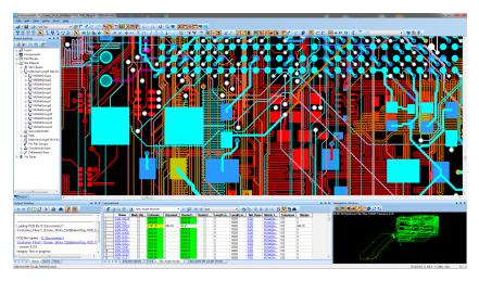
The Advanced PCB Option allows automatic routing of high-speed constraints.
