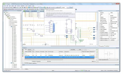
Included in all PADS configurations are intuitive project and design navigation, complete hierarchical support, and advanced tools for design rules and attribute management. Video tooltips ease the learning curve.
