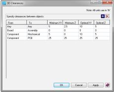
PADS Standard Plus provides 3D design rule checks, based on your PCB design constraints and clearance definitions.
