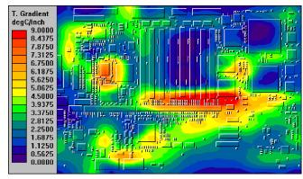
Thermal analysis is available directly from within PADS Standard Plus.
