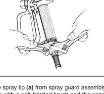
4. Remove spray tip (a) from spray guard assembly. Clean spray tip with a soft-bristled brush and the appropriate cleaning solution. Be sure to remove and clean the washer (b) and saddle seat (c) located in the rear of the spray tip assembly.
