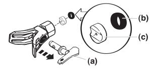
6. Install spray tip (a), saddle seat (c) and washer (b), and replace spray guard assembly.
