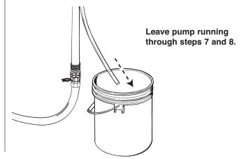
While pulling the trigger, turn the PRIME/SPRAY knob to SPRAY to purge material from the hose back into the original container.
