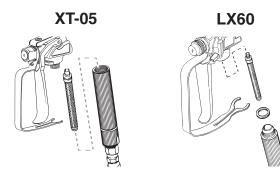
5. Install gun filter tapered-end first. Reassemble spray gun.
