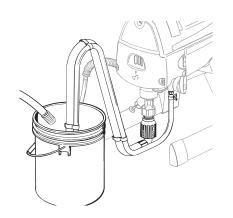
Verify that the seals are present inside the adapter and suction tube (a). Thread the pump cleaning adapter (b) onto a garden hose (c). Connect hose and adapter to the fitting on the end of the suction tube (d).
