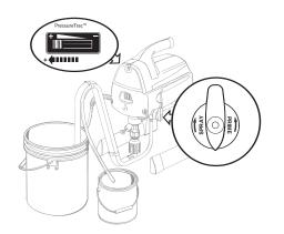
6. Switch the pump OFF (O). Remove the return tube from the waste container and place it in its operating position above the container of spraying material. Use the metal clip to bind the two hoses together.
