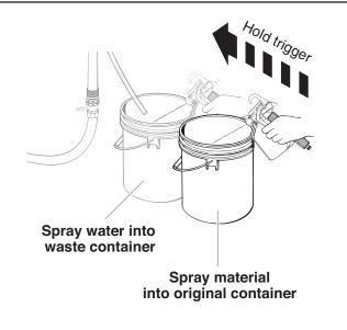
Move on to Cleaning the Spray Gun Components.
