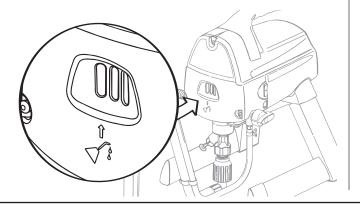
3. Place a full container of spraying material underneath the suction tube (a). Secure the return tube (b) into a waste container.
