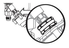
If priming problems persist, you may need to replace the inlet valve assembly. Call Technical Service to order new inlet valve assembly.
