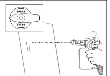
Release the trigger and lock the gun off (see page 7). Reverse the tip so the arrow points forward again (SPRAY position). Unlock the gun and resume spraying.
