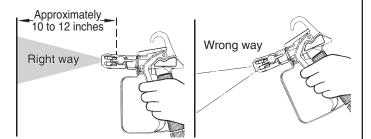
Tip: Trigger gun after starting the stroke. Release the trigger before ending the stroke. The spray gun should be moving when the trigger is pulled and released. Overlap each stroke by about 30%. This will ensure an even coating.
