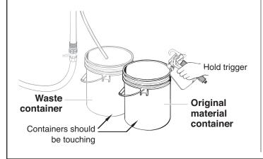
6. Turn water supply on. Turn pump ON (I). Water will go into the suction tube and out through the return tube. Let pump run for a few minutes to allow the return tube to be flushed.
