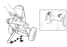
Twist the knob on either side of the cart toward the "UP" arrow until it stops.
