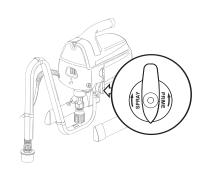
3. Unlock the spray gun and trigger spray gun into the side of the material bucket. Lock the spray gun.
