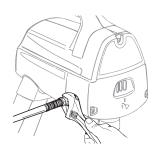
5. Thread the other end of the hose to the spray gun. Hold the gun with one adjustable wrench, and tighten the hose nut with the other.
