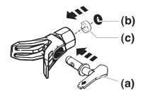
7. Thread the spray gun back onto the paint hose. Tighten with a wrench.
