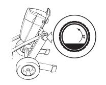
Lift the handle until the motor housing and handle locks into place.
