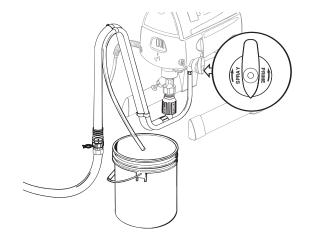
7. Place the original material container next to the waste container. Aim the spray gun into the side of the **original material container** and hold the trigger.
