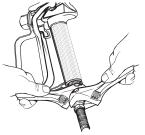
6. Remove cap from inlet valve (a). Thread the suction tube onto the inlet valve and tighten firmly by hand. Be sure that the threads are straight so that the fitting turns freely.
