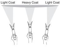
**Tip:** Keep the spray gun perpendicular to the surface, otherwise one end of the pattern will be thicker than the other.
