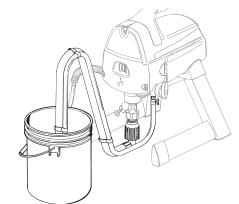
6. Let the pump circlulate cleaning solution through the suction set for 2-3 minutes. Turn the pump OFF.
