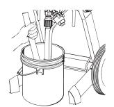
3. Turn the PRIME/SPRAY knob to SPRAY. Test the sprayer on a practice piece and begin spraying.
