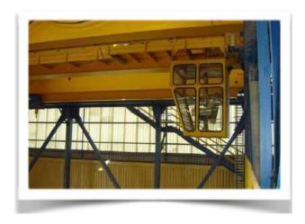
The operator's cabin on the bridge crane itself offers a better view of the loads to be handled and is mainly suitable for handling bulky loads.
