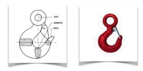
REMEMBER, a hook should not be deformed in an attempt to increase its load capacity. A bent hook must be destroyed.
