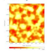
An interferometer image is dominated by the effects of (u, v)sampling.
