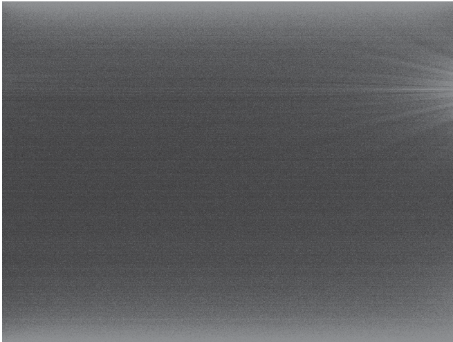
Figure 10. A 120 second dark frame, from a G10. Note the amp glow on the upper right side, this is standard for the ICX294 chip, and is removed from light images during dark frame subtraction. The G16 will show a different dark frame amp glow signature, and the G26/G24 have ZERO amp glow!
