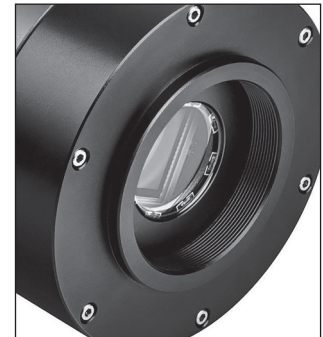
Figure 3b. T-threads for direct threaded connection (G10 and above). StarShoot Mini cameras slip into 1.25" focuser, or use c-mount threads. G24 has larger 54mm opening and includes step down rings
