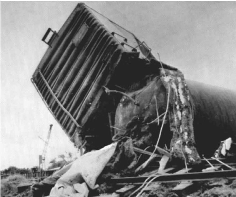
Figure 3.1 Drying cylinder explodes when an almost foolproof safety device failed. (Courtesy of The Hartford Steam Boiler Inspection and Insurance Company.)
