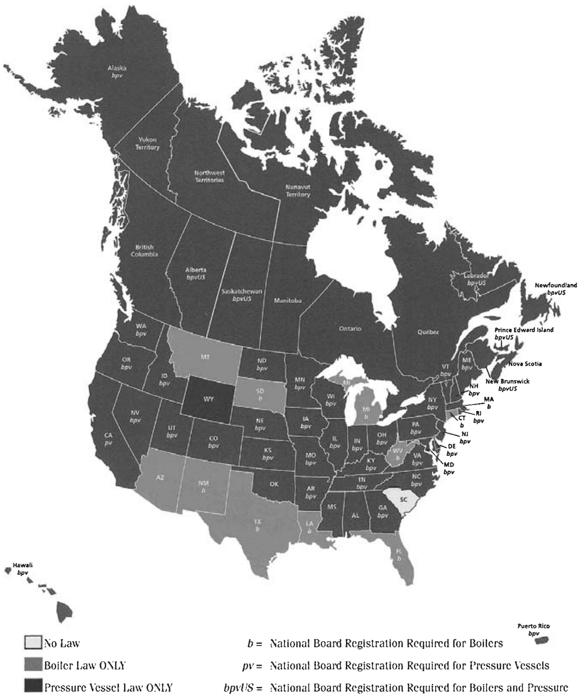
Figure 1.3 Boiler and pressure vessel laws in the United States and Canada. (Reprinted with permission of the National Board of Boiler and Pressure Vessel Inspectors, www.nationalboard.org , from National Board Synopsis of Boiler and Pressure Vessel Laws, Rules and Regulations, © 2003.)
