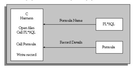
A C code harness performs the file handling (opening, closing and writing to files), and enables the PL/SQL and the formulas to interface.
