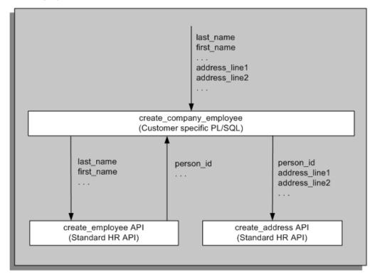
With API user hooks it is not possible to change any of the data values. So the building block approach can be used to default or set any values before the published API is called.
