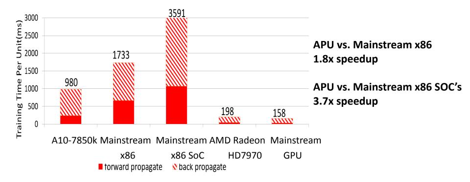
Mini-batch size: 1024 CPU prepares data, GPU computes
