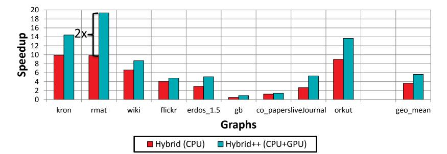
Y-axis represents speedup over the 4-core OpenMP reference BFS algorithm in Graph500
