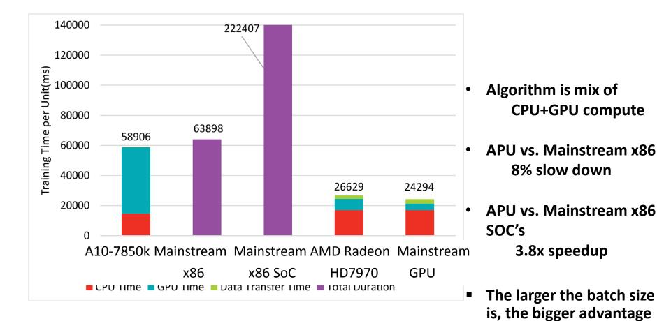
Data: CIFAR10, Mini-batch size: 2048 CPU: L-BEGS: GPU: Autoencoder forward and
