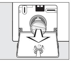
Remove the drain filter completely.
