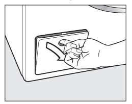
Open the drain pump flap.
