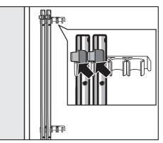
Secure the shipping struts to the back of the washing machine. Make sure that the top catch is located above the holder.
