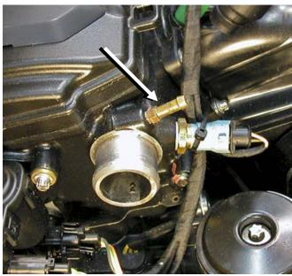
NOTE: Apply pipe thread sealant to threads. Tighten screw until head is flush with cylinder head.
