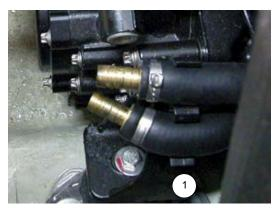
NOTE: Install larger end of splicer into oil cooler hose.
