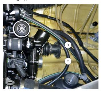
Route cooling line over drive shaft and towards exhaust pipe/water box joint.
