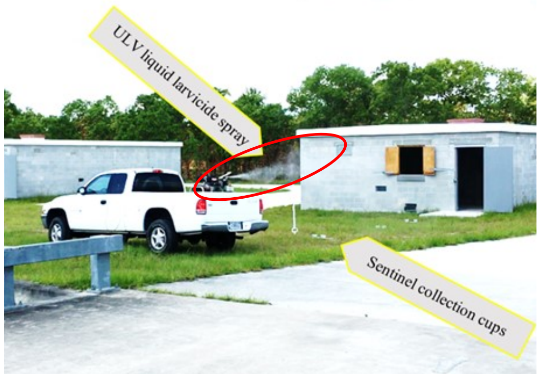
Figure 1. A ULV truck-mounted sprayer applying liquid larvicide while driving along a path outside simulated urban structures, Camp Blanding, Florida. Note plastic cups placed on the ground to collect droplets of sprayed larvicide for later lab tests to observe frequencies of mortality in Ae. aegypti larvae. These cups were placed at increasing distances from the sprayer, through the inside of the building, and outside to the rear of the building. This experimental larvicide spray application represents one control method used in neighborhoods infested with Ae. aegypti mosquitoes in dengue-endemic regions, and the placement of sentinel cups reflects the challenge of reaching cryptic habitat throughout a residential property with access only from the street.
