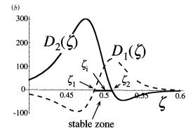
**Figure 2.** (a) Field on the axis inside a solenoid with  $\delta = 2a/L = 0.1$ ; (b) the discriminants  $D_1(\zeta)$  and  $D_2(\zeta)$  defined by (16), and the stable zone where both are positive.
