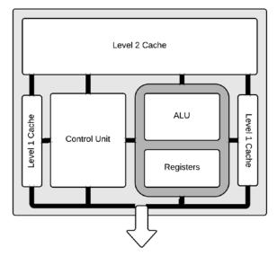
The CPU contains a **control unit**which coordinates the timing of the units and the flow of data in the CPU. It is responsible for fetching and decoding instructions and also managing their execution on the processor.
