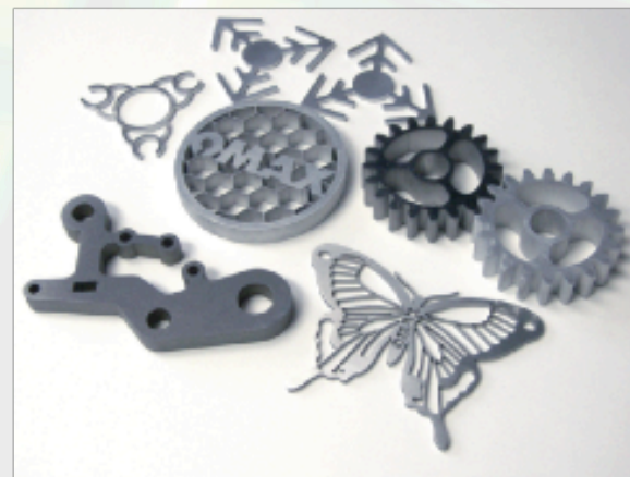
FIGURE 9.38 (a) Schematic illustration of water-jet machining. (b) A computer-controlled water-jet cutting machine. (c) Examples of various nonmetallic parts machined by the water-jet cutting process. Source: Courtesy of OMAX Corporation.
