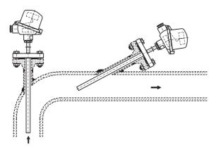
Figure 6: Classic installation of temperature sensors in piping
