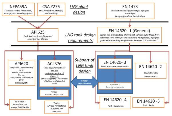
The suggested way to incorporate the Membrane tank system into NFPA59A, which was also the CSA 276 committee adopted, is to consider the same Sub-standard for Membrane tank systems (NFPA59A $\rightarrow$ API625 $\rightarrow$ ACI376+API620) for all common components, and to refer to European Std for parts which are exclusive to the Membrane system (NFPA59A $\rightarrow$ API625 $\rightarrow$ EN14620).
