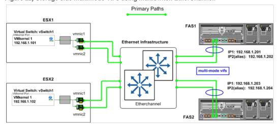
Figure 22) Storage side multimode VIFs using multiswitch EtherChannel.
