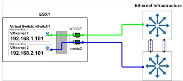
Figure 39) ESX server physical NIC connections with traditional Ethernet.
