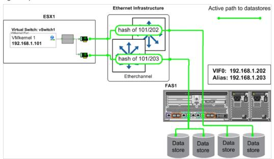
Figure 23) Datastore connections with multiswitch EtherChannel.
