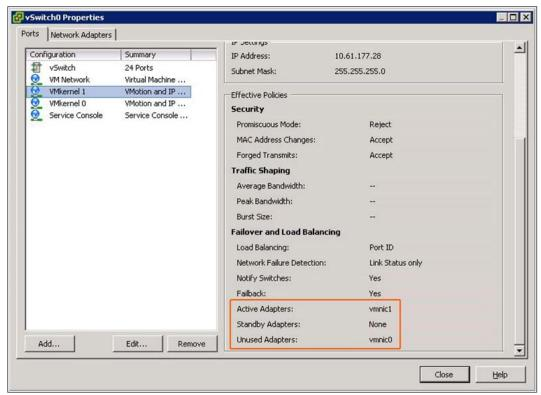
Figure 44) iSCSI to VMkernel bindings for use with multiple TCP sessions.
