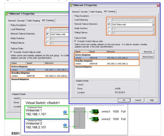
Figure 40) ESX server VMkernel port properties with traditional Ethernet.
