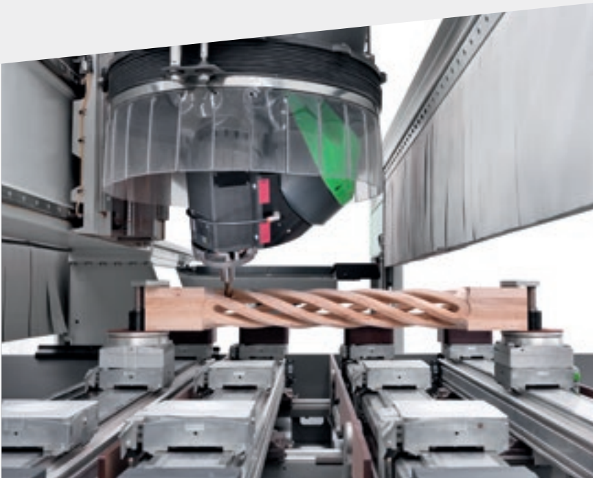
5-axis milling unit with 360mm hood with adjustable height.
