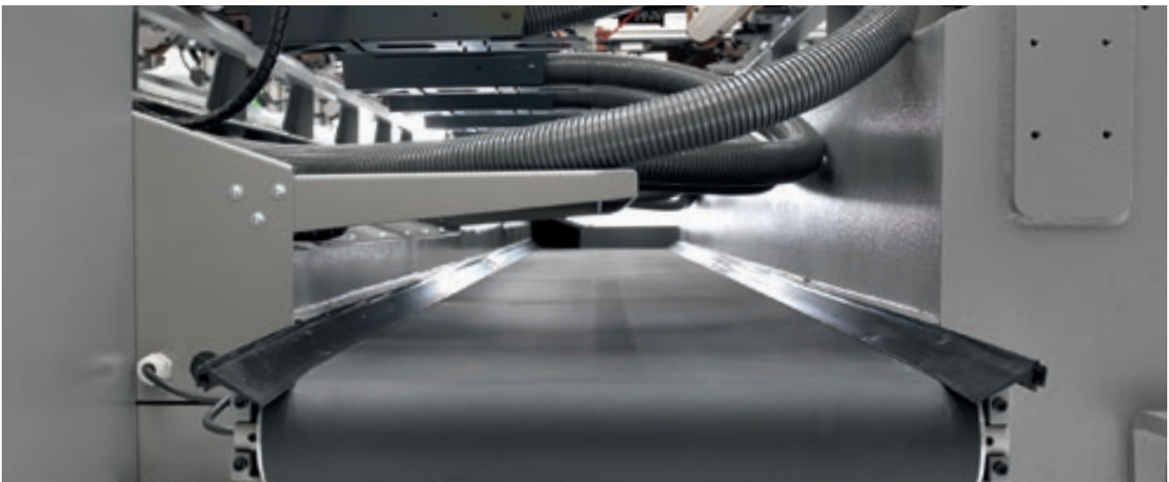
Motorised conveyor belt for the removal of chips and waste.
