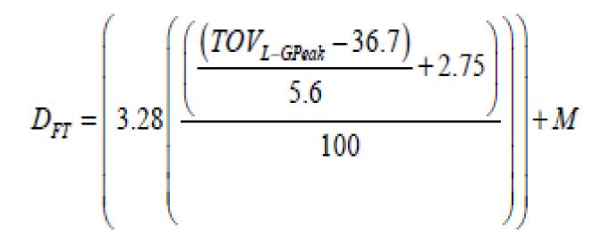
MAD, line-to-line, for line-to-line voltages equal to and less than 242 kV
