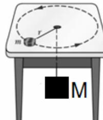
22. A heavy (2.0 kg) point-like object rests 2.0m from the center of a rough turntable as the turntable rotates. The period of the turntable's rotation is 5.0 seconds. The coefficient of kinetic friction between the object and turntable is 0.50, while the coefficient of static friction is 0.80. What is the magnitude of the force of friction acting on the object?
