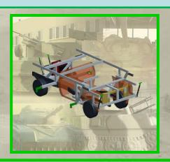
LCM consists of an unmanned host chassis integrated with a full-scale plastic target façade. The common support structure supports a variety of full-scale plastic surrogate targets.
