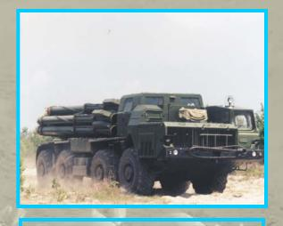
Actual SMERCH MRL MAZ-543 chassis with fabricated firing cab and rocket launcher
