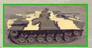
The BMP3-S emulates the threat infrared (IR), millimeter wave (MMW) radar and visual signatures of the threat within a wide range of environmental conditions.
