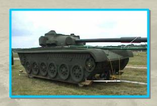
A full-scale, validated, plastic surrogate target that replicates a T-80 Main Battle Tank in its magnetic and electro-optical signature
