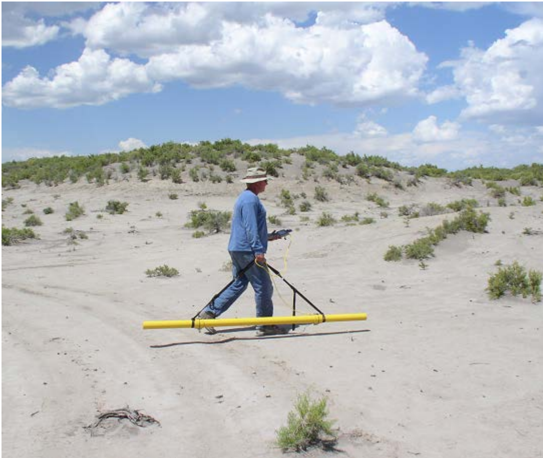
Photo 1. Alan Stuebe, MLRA Project Leader, USDA-NRCS, Alamosa, CO conducts an EMI survey with the DualEM-2 meter in an area of Corlett-Hooper complex within the lake bed area of Ancient Lake Alamosa . The Corlett soils component (observed in the background) is associated with sandier textures and dune-like topography.
