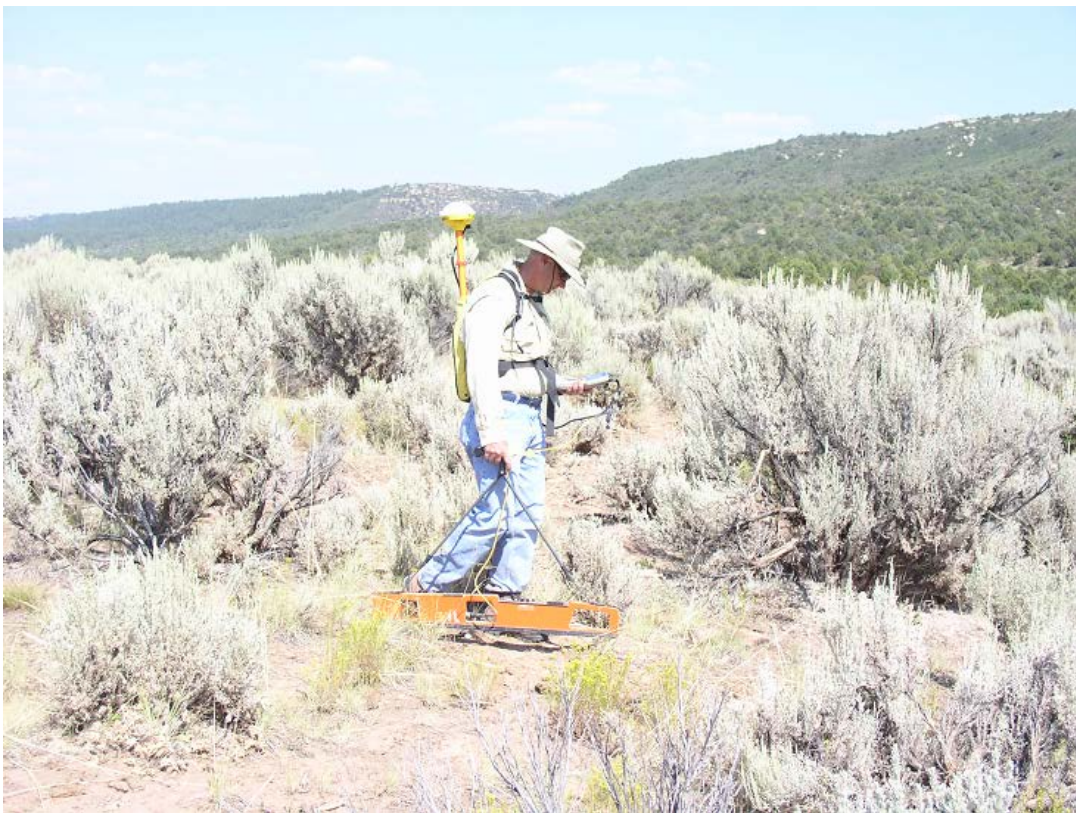
Photo 3. Wes Tuttle, Geophysical Soil Scientist, USDANRCS/NSSC, Wilkesboro, NC completes an apparent conductivity survey with the Geonics EM38 meter in an area of Weatherill loam, 3 to 6 percent slopes at the House Creek Village site.
