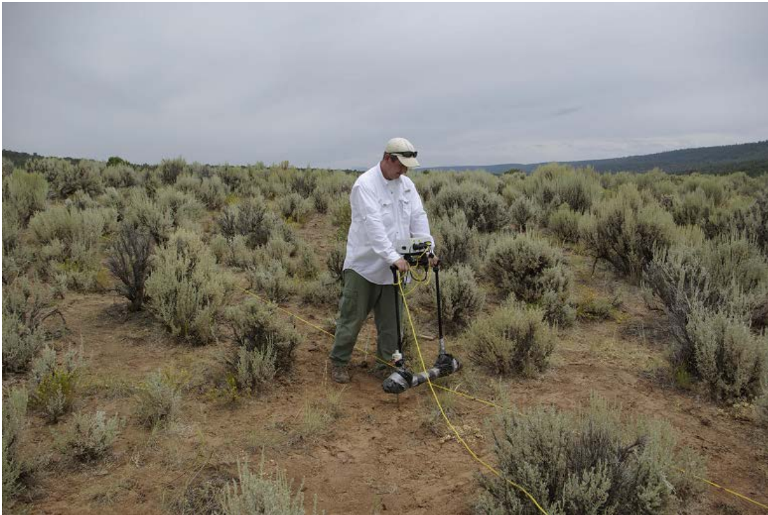
Photo 4. William (Bill) Volf, Archaeologist, USDA/NRCS, Cortez, CO completes a resistivity survey at the House Creek Village site. Bill is using an RM-15 resistivity meter manufactured by Geoscan Research.
