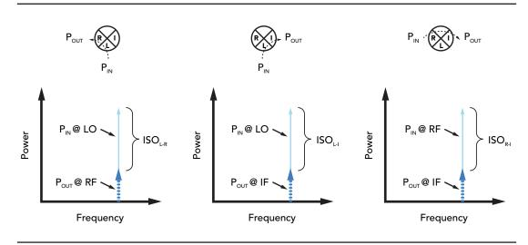
Figure 8: Definitions of mixer isolation for L-R, L-I and R-I isolation.
