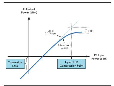
Figure 9: Graphical representation of 1 dB compression point.
