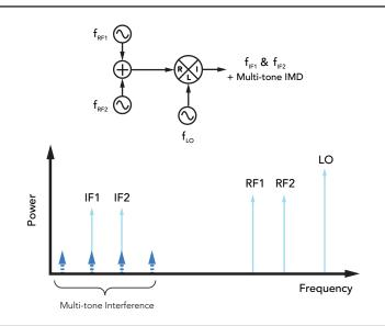
Figure 12: Illustration of multi-tone IMD created by two closely spaced RF signals. Generated IMD tones overlap with desired IF<sub>1</sub> and IF<sub>2</sub> signals.
