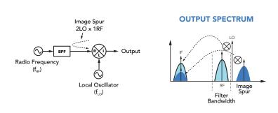
Figure 10: Schematic diagram (left) showing backreflected 2LO x 1RF spur from reactive bandpass filter (BPF). Output spectrum (right) showing desired IF and downconverted image spur overlapping in frequency.
