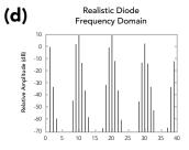
Figure 3: Time and frequency domain comparing the output of the single ended mixer in Figure 2 with ideal and relatistic diode switching characteristics.
