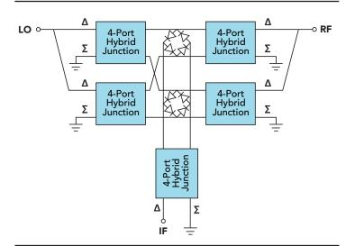
Figure 7: <u>Doubly double balanced mixer</u> (aka triple balanced mixer).
