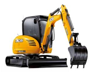
The JCB 8040 ZTS, 8045 ZTS and 8050 RTS/ZTS feature a 34kW (46hp) engine, making these machines very powerful for this class of excavator.
