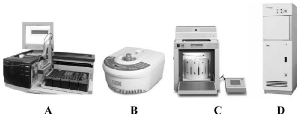
Fig. 4. Microwave reactors for chemical syntheses. A: Emrys Liberator (Biotage, Sweden, www.biotage.com ); B: CEM Discover BenchMate (CEM, USA, www.cem.com ) Copyright CEM Corporation; C: Milestone Ethos TouchControl (Milestone, Italy, www.milestonesci.com ); D: Lambda MicroCure2100 BatchSystem (Lambda, USA, www.microcure.com ). With permission.
