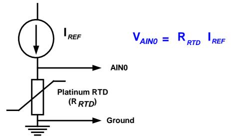
RTD's require a constant current source, such as 1mA. Such a low current keeps the self heating to a minimum.
