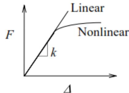
$k = F / \Delta$  ( $> 0$ ) is the force needed to produce a unit stretch.
