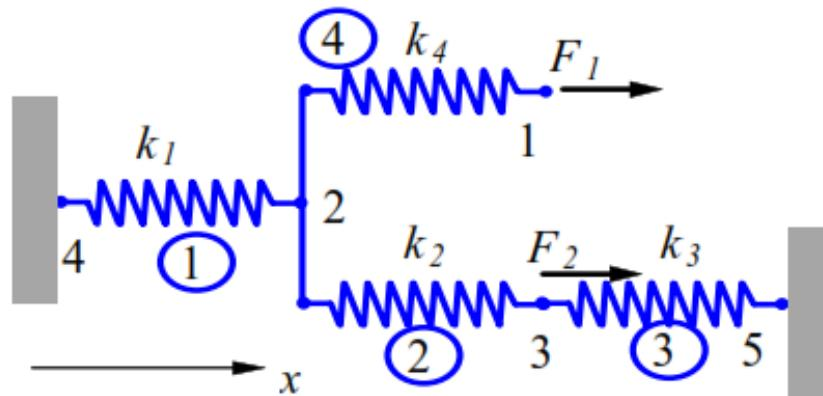
**Problem:** For the spring system with arbitrarily numbered nodes and elements, as shown above, find the global stiffness matrix.
