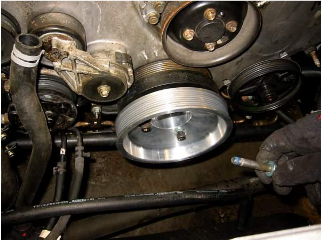
Attach crank blower pulley to crank pulley
