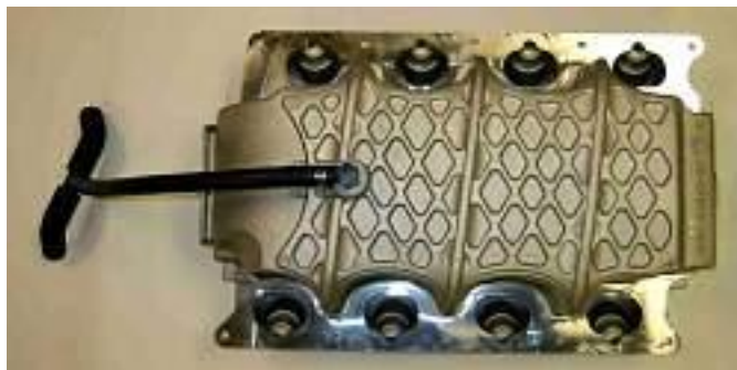
PCV Hose Assembly plugged to Lower Intake Manifold
