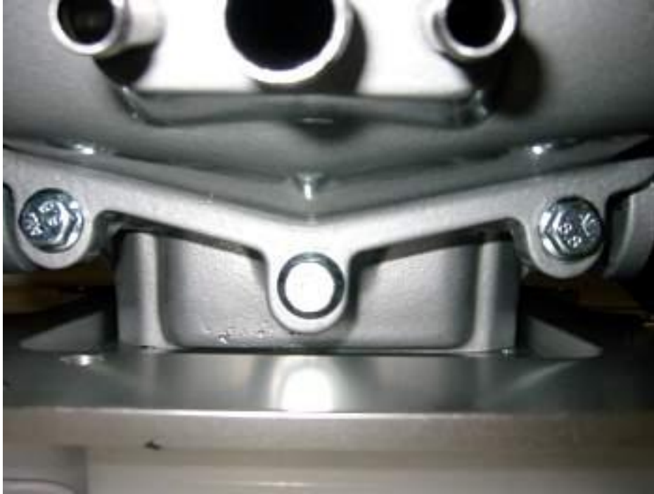
Back view of Inlet Duct assembled with Blower
