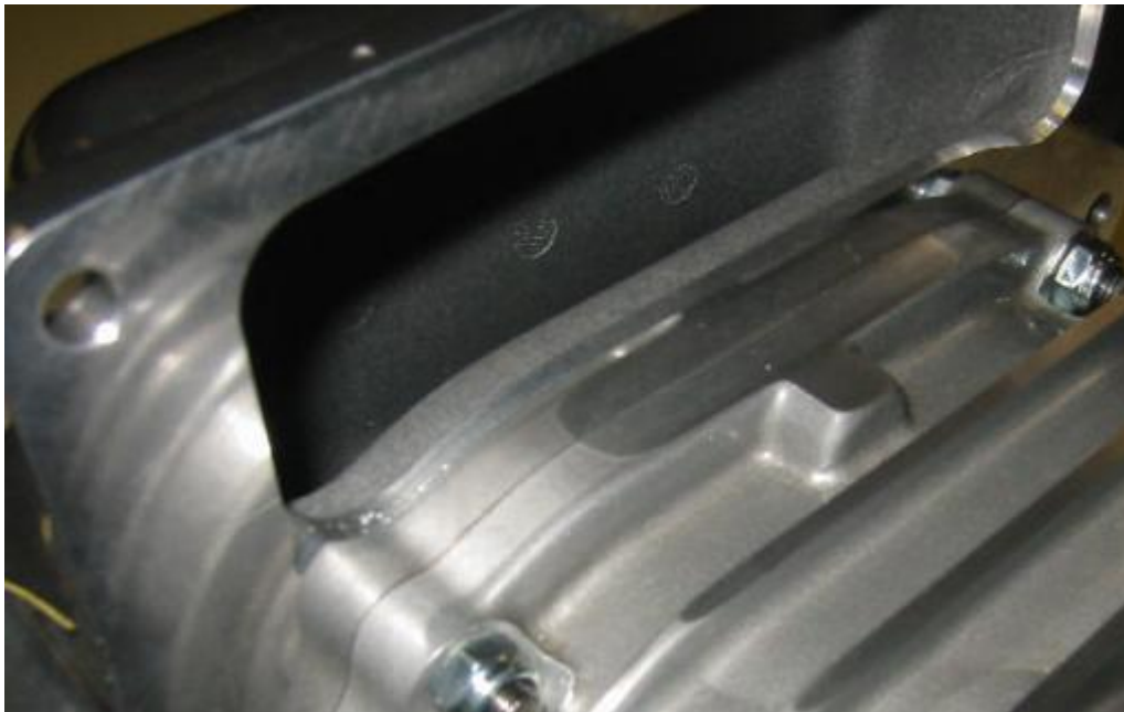
Front view of Inlet Duct assembled with Blower
