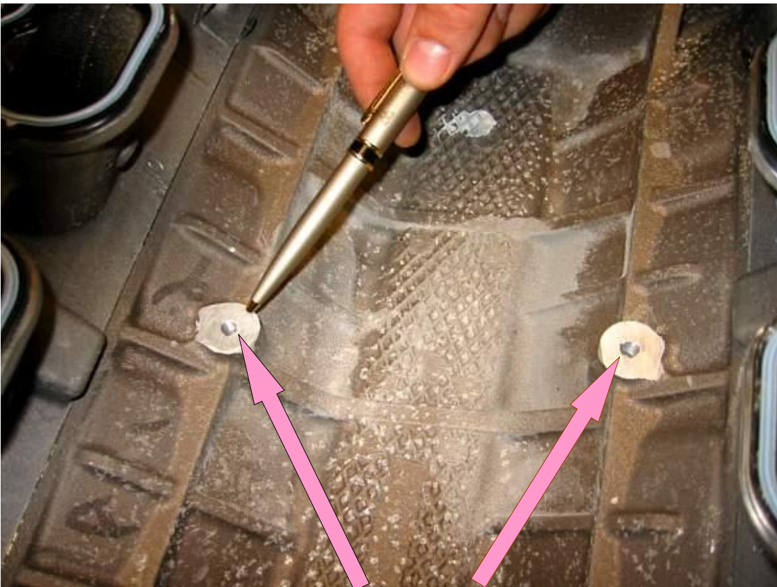
Knock sensor bosses after grinding
