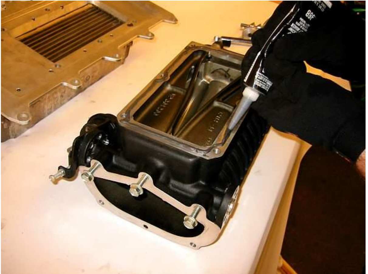
Silicon seal on blower
