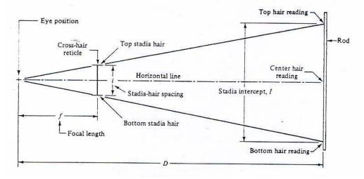
The distance between the top and bottom stadia hair is identified as i (stadia hair spacing). The distance between the top and bottom reading on the rod is identified as I (stadia intercept). The distance from the instrument operator's eye to the stadia reticle (eyepiece) is identified as f (focal length). The distance from the instrument operator's eye to the level rod is identified as D, which is the quantity being determined in a stadia survey. From similar triangles
