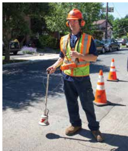
Leak detection equipment has helped over 2,000 residents save water and money
